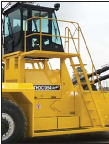
Anti-slip steps and handrails for 3-point mounting and dismounting (meets new proposed ANSI B56.1 standard)
